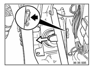
Disconnect return spring for brake pedal. Take off locking clip for shaft pin of brake pedal. Push out shaft pin.
