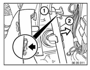
Take off locking clip (1) for brake pedal. Pull off brake pedal (2).
